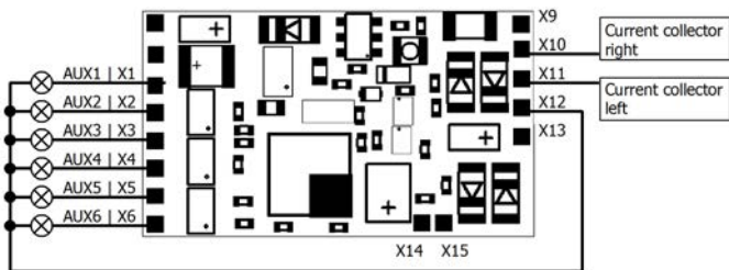
Fig. 1: Connection of the voltage supply and of accessories
