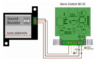
3.1. Connection to the SD-32 servo control module
