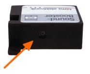
The housing of the sound-booster has a hole on the back behind which the trim pot for adjusting the volume is located. Use a small screwdriver to adjust the volume.
