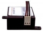
Plug the socket strip onto the pin header of the sound-booster and make the connections to the control module (SD-32 servo controller or LC-NG module) according to the connection diagram and the table.
