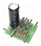
Switching amplifier for points with double solenoids
