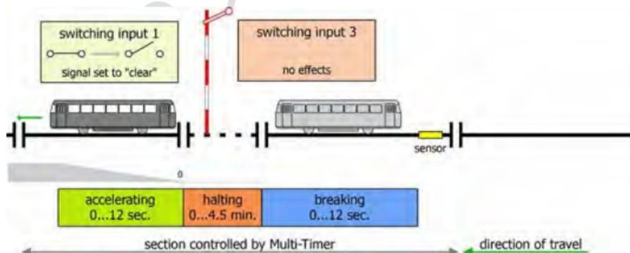
**Example 2: Signal set to "Clear"** (switching input 1 open)
