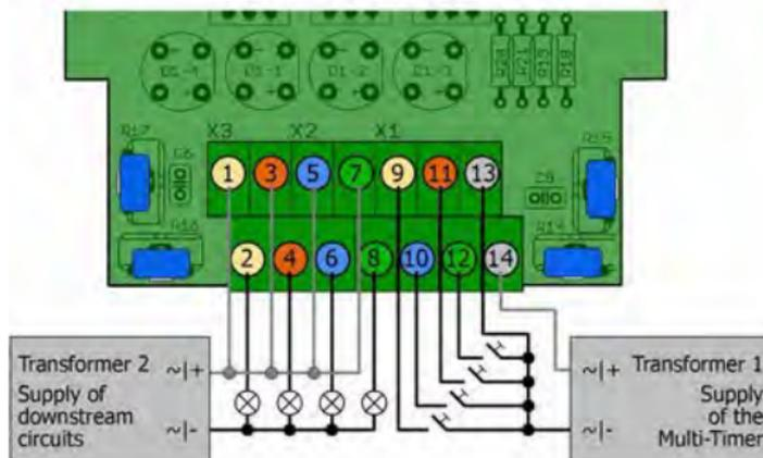
Choose operation mode 1 (r) for testing all outputs, so do not insert a jumper to any of the solder pins (→ section 8). Set a short switching time (trim-pot as far as it will go to the left). Then check all four outputs and switching inputs one after the other.
