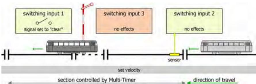
Passing the sensor at the beginning of the braking track has no effect, the braking process is not started. The state of switching input 3 has no effects, too.
