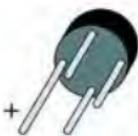
Rectifiers convert alternating into direct voltage. They have four pins: two for the input voltage (a.c. voltage) and two for the output voltage (d.c. voltage). The pins for the output voltage are polarized.
