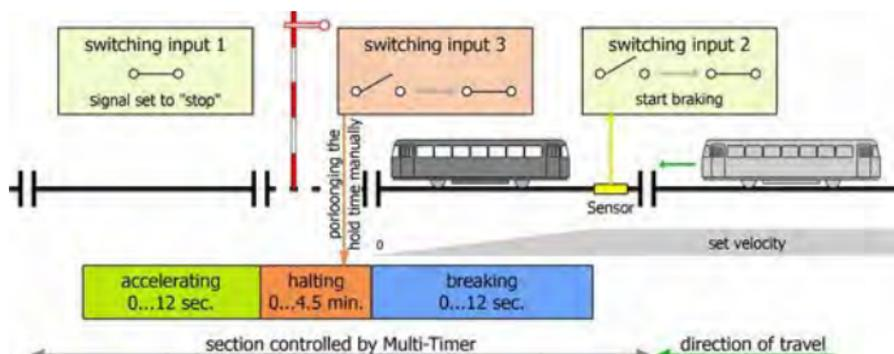
2. The locomotive stops in front of the signal until the hold time has expired (and switching input 1 has been switched to "open" automatically) or until switching input 1 has been opened (e.g. by means of an external switch).
