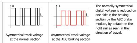
In principle, the braking section is only effective for one direction of travel at a time. When travelling in the opposite direction, the locomotive does not react to the braking section.
