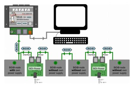
In the example, a BiDi-Power module supplies nodes 2 and 3 and another BiDi-Power node 4. Before the first BiDi-Power module, a node with its own power supply is connected to the BiDiBus.
