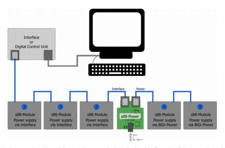
In the example, s88 modules 1 to 3 are supplied via the bus line from the digital control unit / interface. The current that the control unit / interface can provide for the s88 bus is not sufficient to supply further s88 modules. A s88-Power is therefore inserted into the bus line. This supplies 700 mA current for the supply of further s88 modules (here s88 modules 4 and 5).
