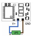
Connection of a buffer circuit that can be used without connecting a control line (e.g. UPS-mini)
