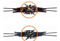
In this case, adjust the wire brackets on the top and/or bottom of the couplings CAREFULLY with a small pair of needlenose pliers until they touch.
