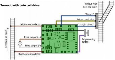
Tip: If the turnout switches contrary to the turnout setting commands entered, you can swap the turnout setting by changing the CV settings ( $\rightarrow$  CV5).
